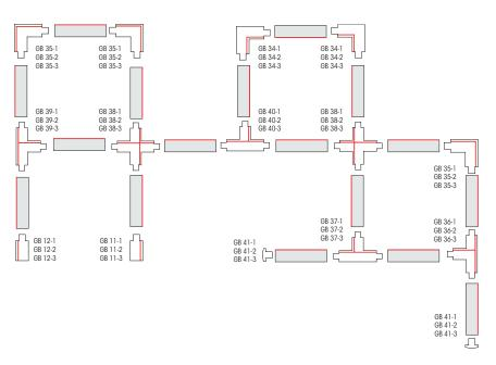
Diagram above shows the use of L-, T- and X- Feed. Red line marks the polarity ridge. Available colours: -1 grey (RAL 7040), -2 black (RAL 9005), -3 white (RAL 9016).
